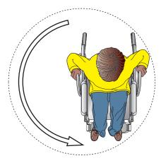
Figure 1. A turning circle for wheelchairs<sup>5</sup>
