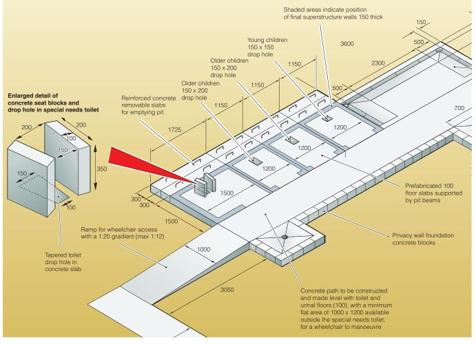
Figure 2. Floor construction: cement block or burnt brick with concrete slab (boys) <sup>9</sup>
